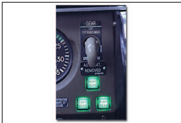
Figure 11-6. Typical landing gear switches and position indicators.
