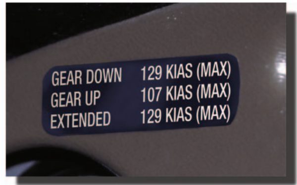
Figure 11-11. Placarded gear speeds in the cockpit.
