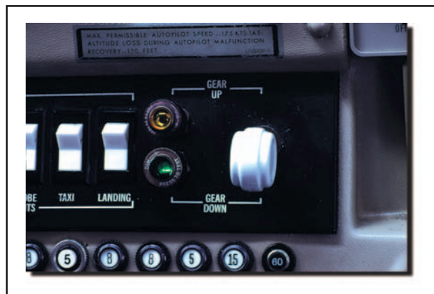
Figure 11-7. Typical landing gear switches and position indicators.
