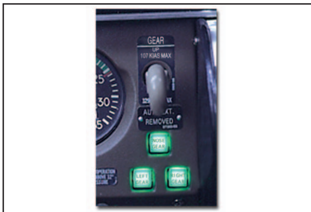
Figure 11-6. Typical landing gear switches and position indicators.
