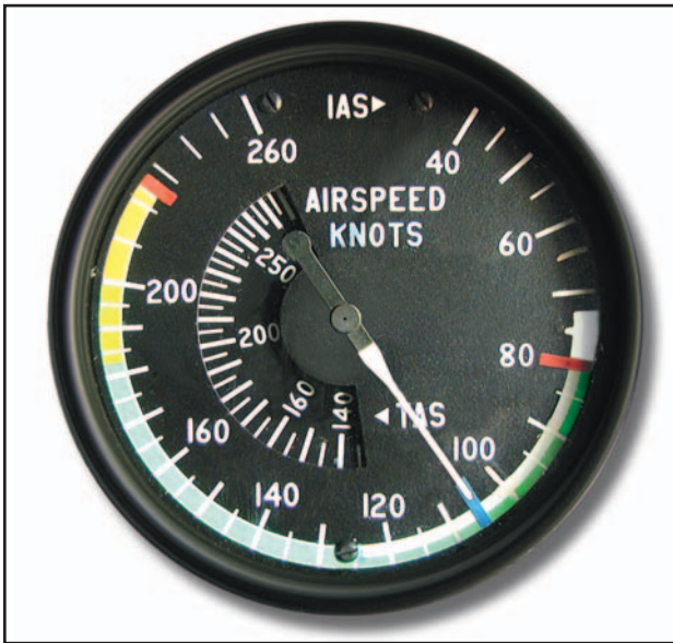
Figure 12-1. Airspeed indicator markings for a multiengine airplane.
